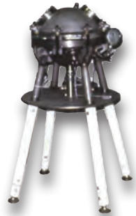
20-Liter Vessel – Used for K_{ST} and P_{MAX} determination
