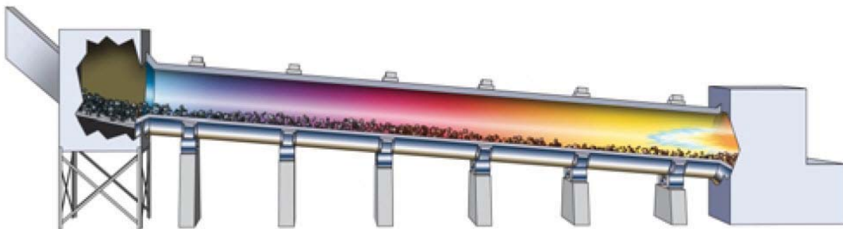
Figure 1: Typical Cross-Sectional View of a Cement Kiln
