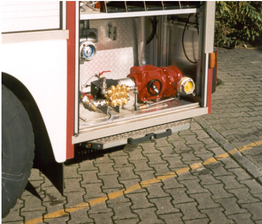
(pict. 1) FireDos ® FD1000/0,3-3-APP-F main water flow: 100-1000 l/min admixture rate: 0,3-3 % step less adjustable operating pressure: max. 16 bar installed in a HTLF 16 of the fire brigade of the town Ulm
