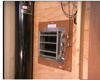
Blade Positions at Peak Pressure of 251 PA. As shown on SHX 300 GD2 data logging sheet. At 13:48:29.845
